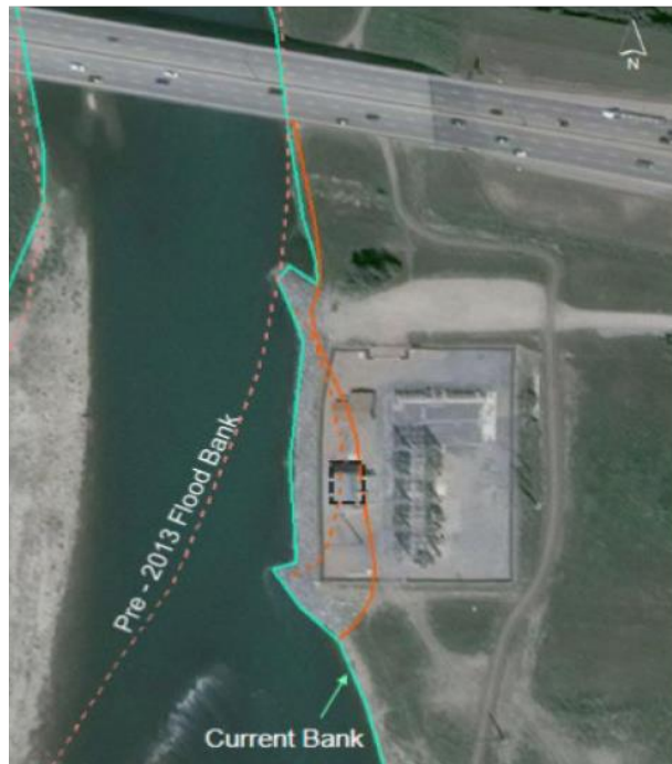
Figure 2. Current and pre-2013 bank at No. 32 Substation 2
