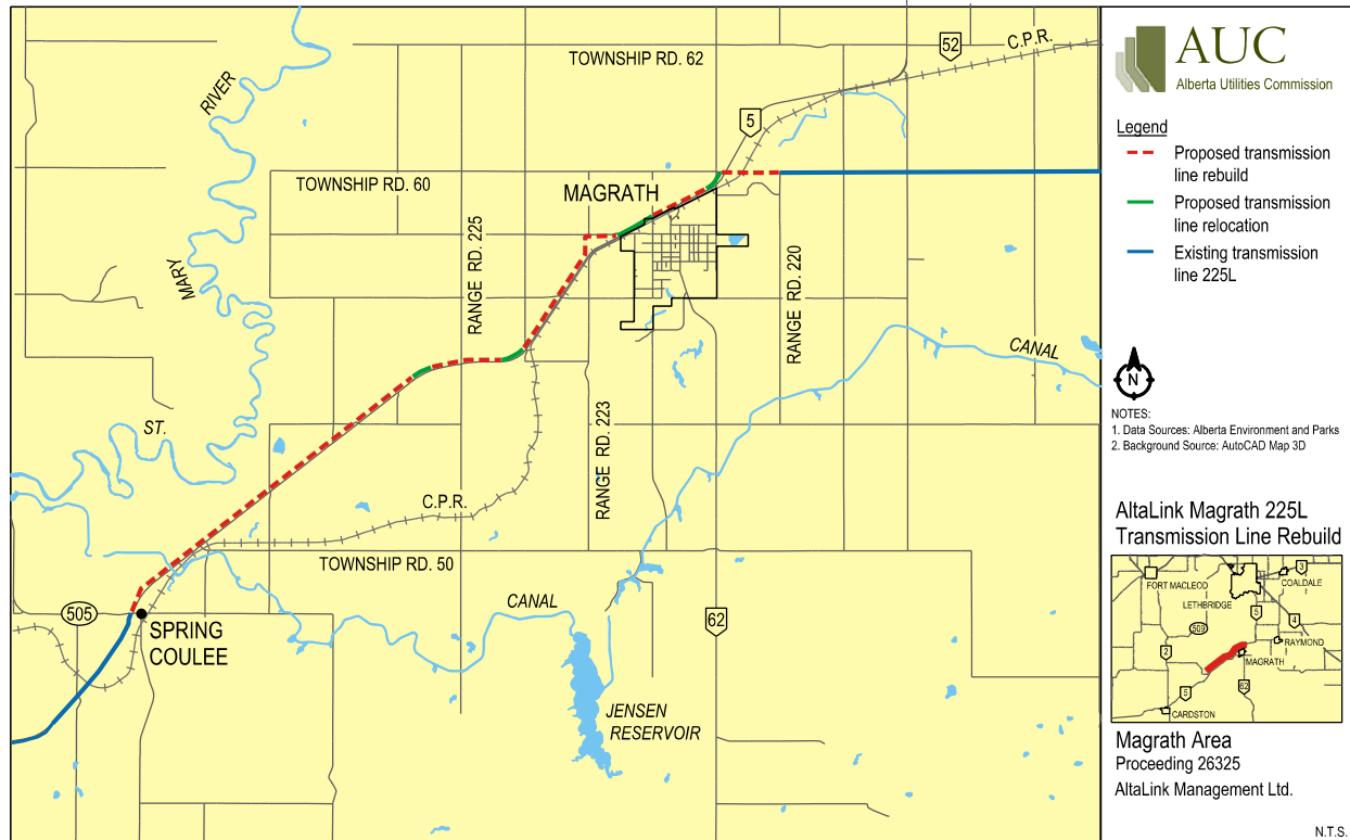
Figure 1. Proposed Transmission Line 225L Rebuild location
