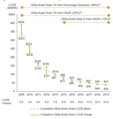
Figure 2. Historical cost of utility-scale solar PV<sup>20</sup>
