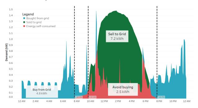
Figure 6. Flows of energy for a small micro-generation self-supply with export customer: from the customer's point of view
