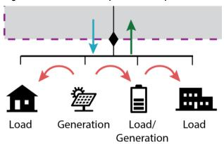
176. Due to these properties, microgrids exhibit the three flows of energy (consuming, self-supplying, and exporting electricity) both *within* the microgrid, as it serves the electricity needs of its members, and *outside* of the microgrid as it interacts with the electric distribution system. Thus, microgrids can be thought of as a self-supply with export configuration with additional attributes due to energy flows between generation and load *within* the microgrid.
