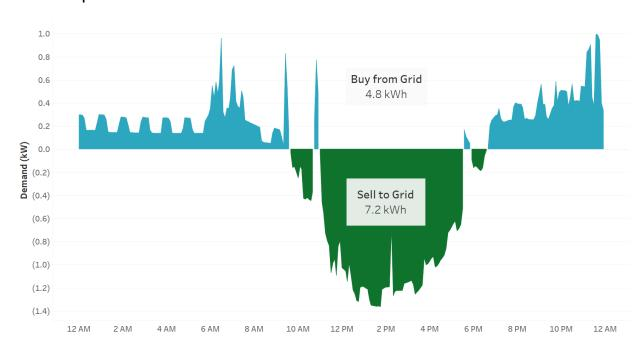
Figure 7. Flows of energy for a small micro-generation self-supply with export customer: from the utility's point of view<sup>45</sup>
